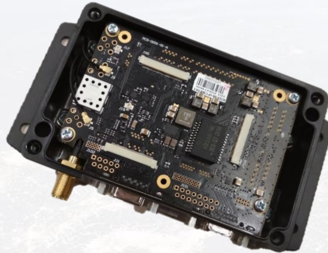
Detail on carrier board hosting the COTS SDR Module
